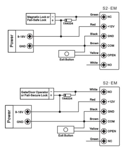
**Attention**: Install a 1N4004 or equivalent diode is needed when use a common power supply, or the reader might be damaged. (1N4004 is included in the packing)
